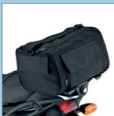
Softcase water resistant synthetic material, 22 l volume, integrated rain cover
